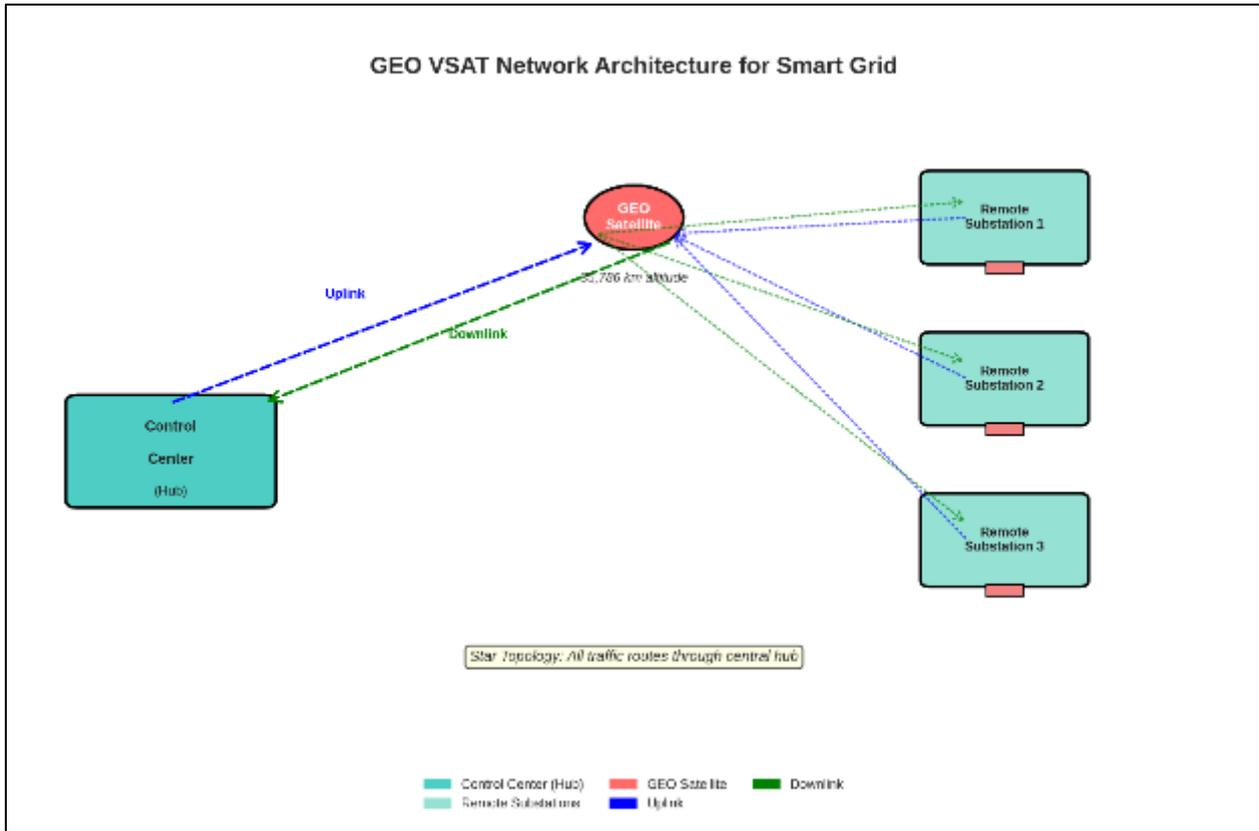
**Figure 1** GEO VSAT Network Architecture for Smart Grid Applications
