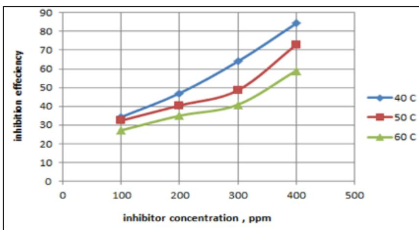
**Figure 4** Efficiency and concentration of the influencer at different temperatures
