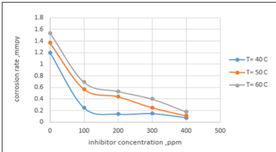
**Figure 8** Corrosion rate and inhibitor concentration at varying temperatures
