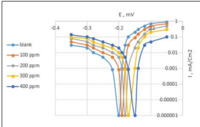
**Figure 1** Inhibitor concentration effects on polarization profiles in an acidic medium at 40 °C
