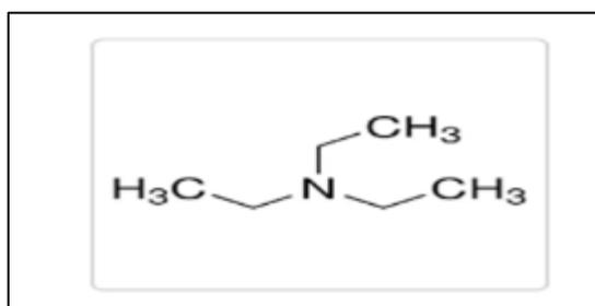
**Figure 11** Tri-ethylamine's chemical composition is  $N(CH_2CH_3)_3$
