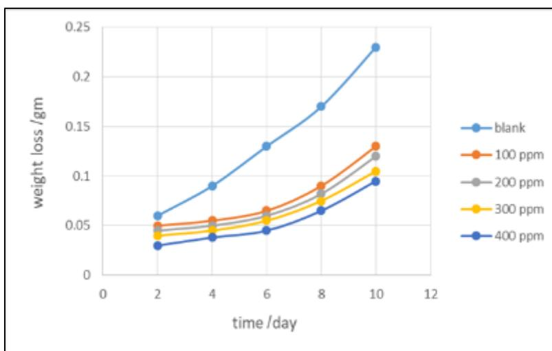
**Figure 5** Effects of different inhibitor concentrations and duration at 40 °C on weight loss
