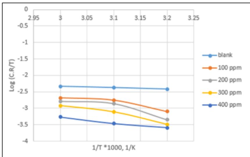
Figure 10 A plot of inverse temperatures (1/T) vs log (C.R./T) at different inhibitor concentrations
