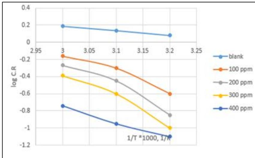
Figure 9 A plot of inverse temperatures (1/T) vs log (C.R.) at different inhibitor concentrations
