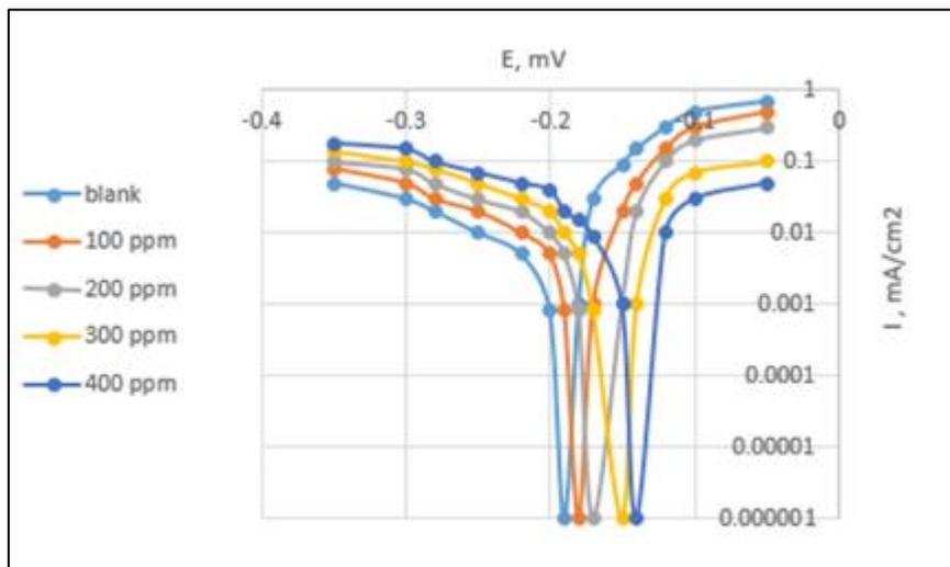
**Figure 2** Inhibitor concentration effects on polarization profiles in an acidic medium at 50 °C
