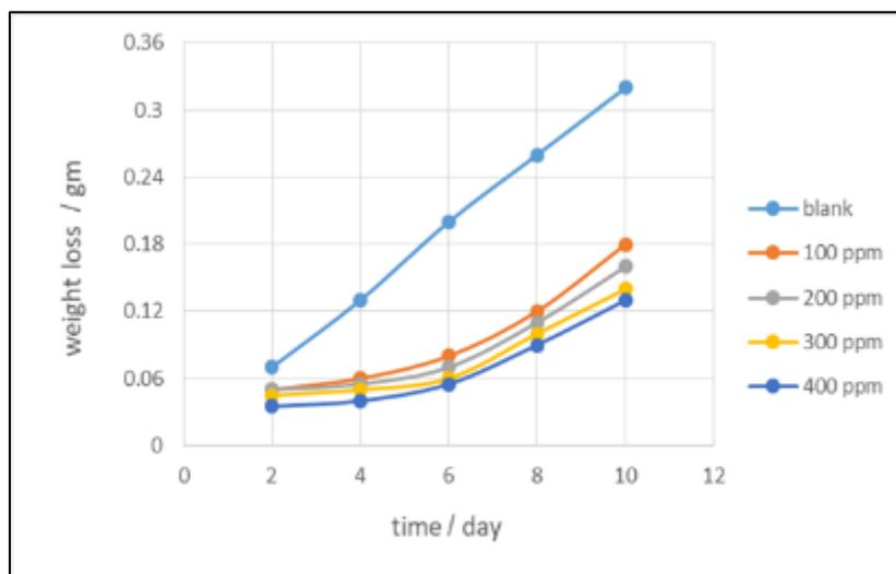
**Figure 6** Effects of different inhibitor concentrations and duration at 50 °C on weight loss
