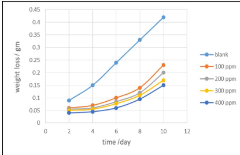
**Figure 7** Effects of different inhibitor concentrations and duration at 60 °C on weight loss
