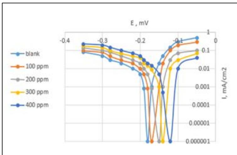
**Figure 3** Inhibitor concentration effects on polarization profiles in an acidic medium at 60 °C
