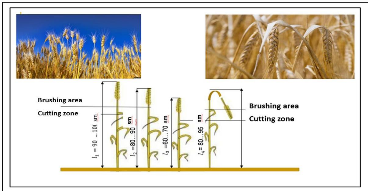
**Figure 1** Dimensions of the height of the wheat stalk and cutting zones
