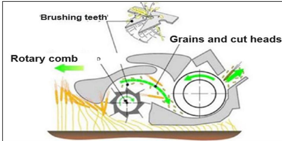
**Figure 2** Technological scheme of a comb-type sickle
