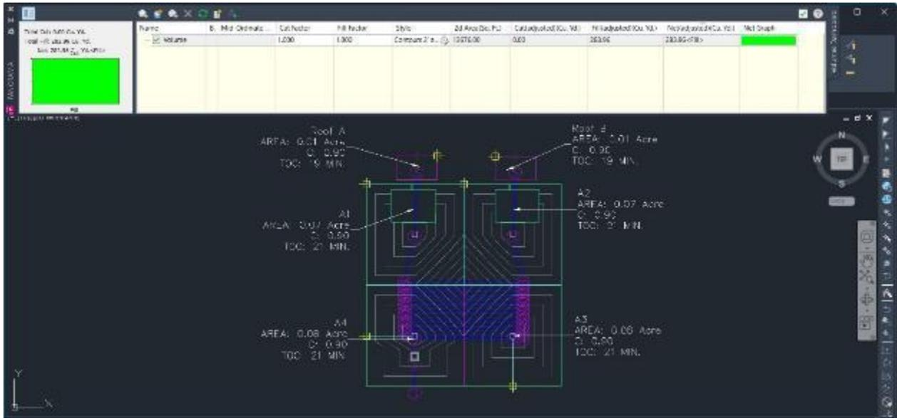
**Figure 8** Catchments and Detention Volume (Civil 3D)
