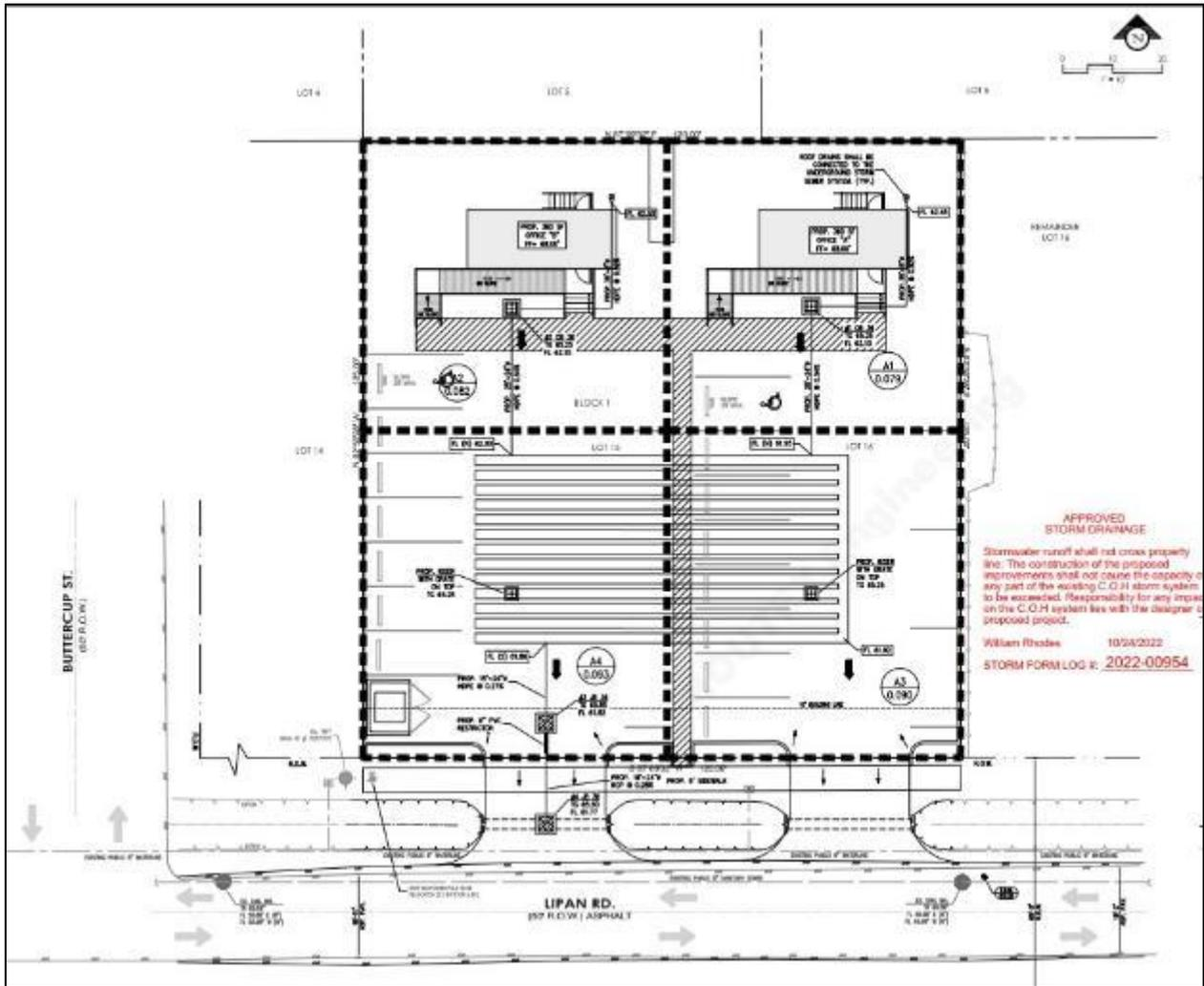
Figure 1 Approved 2022 Houston site plan illustrating the grading layout and underground detention system
