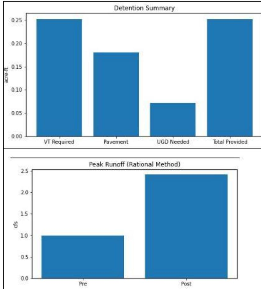
**Figure 7** The Detention Summary chart shows the required and provided storage volumes (acre-ft), while the Peak Runoff chart compares pre- and post-development discharges based on the Rational Method
