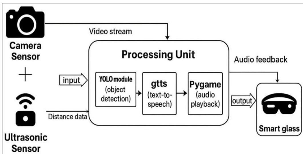
Figure 1 System architecture showing the integration of camera and ultrasonic sensors
