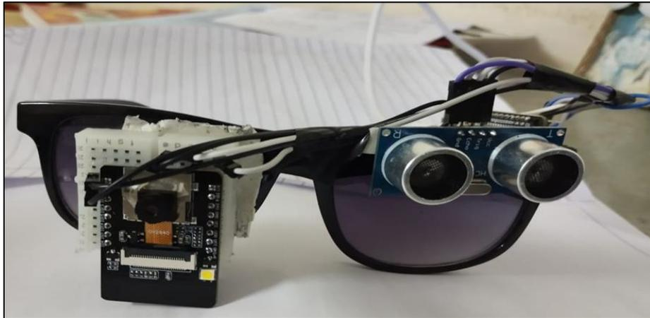
**Figure 2** Physical prototype of the proposed wearable navigation aid
