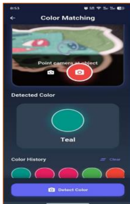
Figure 5 The color matching screen that detects and identifies colors through the camera, helping users coordinate clothing or objects with audio feedback about detected colors
