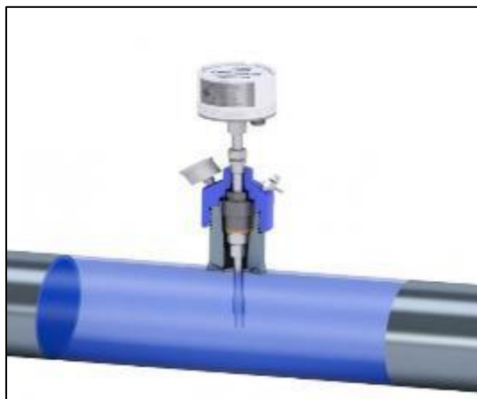
Figure 2 Schematic of a Typical Corrosion Probes Utilized in the Process
