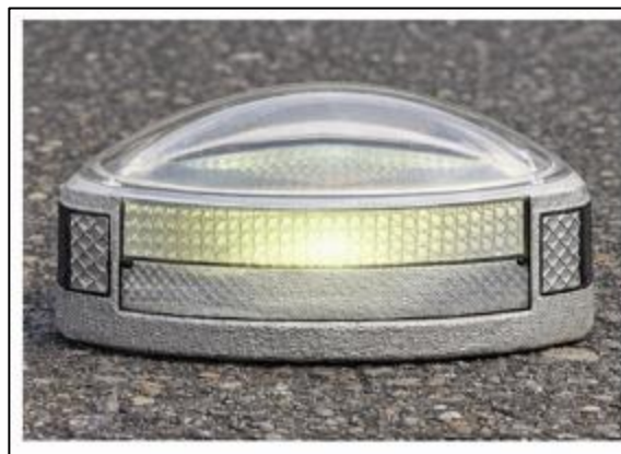
Figure 3 Final fabricated photoluminescent-reflective cat's eye road stud prototype for tropical urban roads
